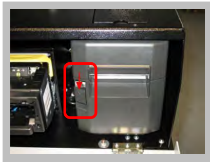
Open the printer by pushing the release mechanism on the left of the printer
