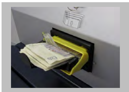
Place the notes in to the bezel, level edge first. The i-Deposit will automatically start to count
